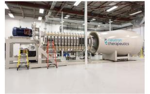
(i) the accelerator can be utilized as a high current DC proton machine. (ii) it can be configured as a high-flux DC neutron source, and (iii) it can be set-up as a multi-ion DC accelerator. For more information, please contact morgan@d-pace.com
