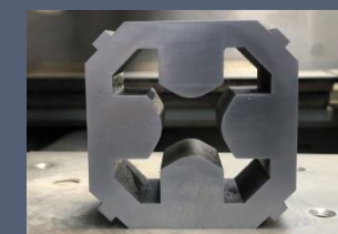
Another example of precision pole tips shaped by wire-cut EDM.
